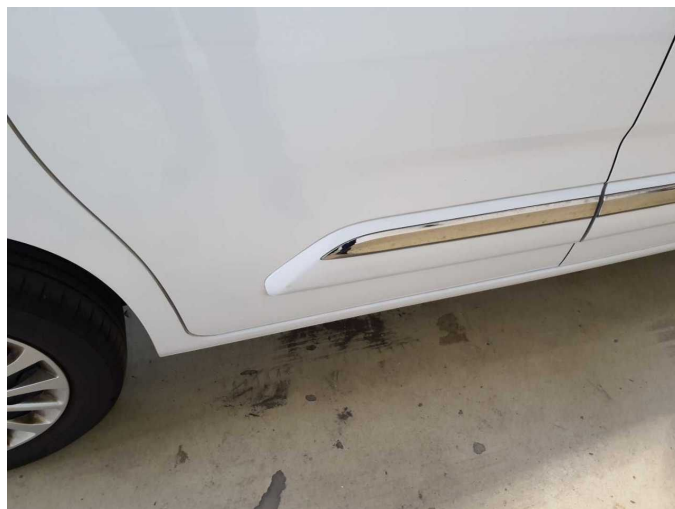
Damage 4: Door - rear right side: Brightware - lower - Scratch(es) - Loss in value
