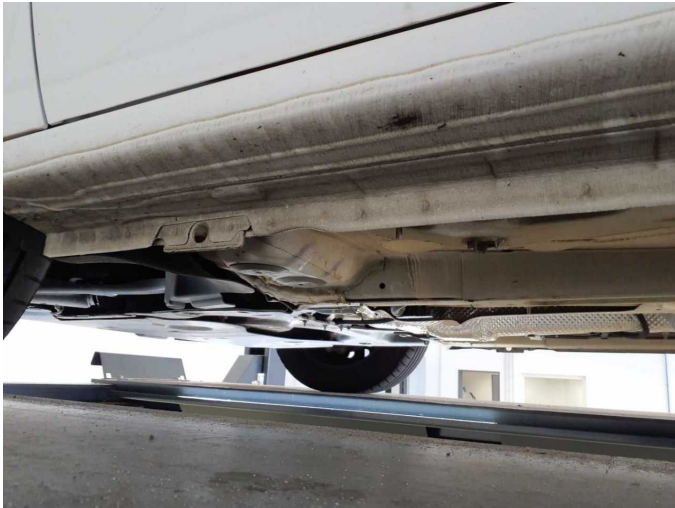
Damage 7: Sill - left side: Sill - dent(s) - Smart repair
