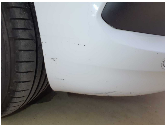
Damage 11: Front bumper: Front bumper (Inklusive anbauteile) - Dent / paintcoat damage - Repair and paint
