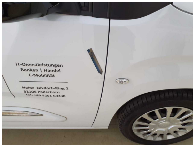
Damage 9: Door - front right side: Door - Dent / paintcoat damage - Smart repair
