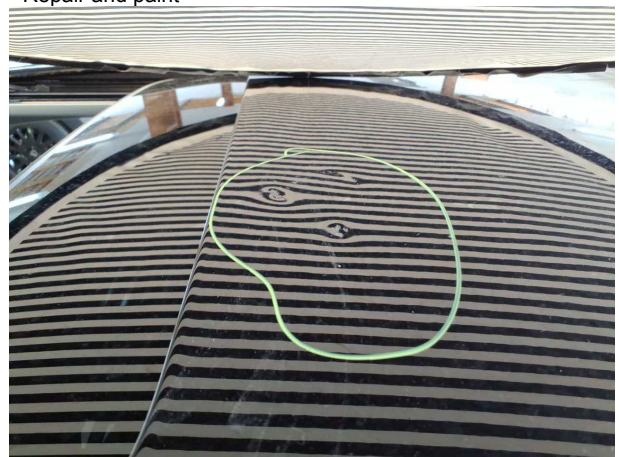
Damage #9: Roof: Roof - Dent / paintcoat damage - Repair a...
