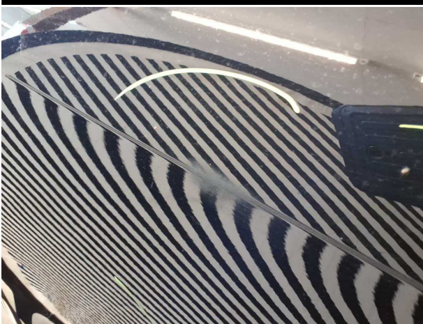
Damage #7: Door - rear right side: Door - Paint defect - Repair and paint
