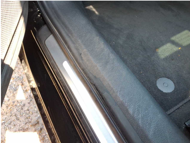
Damage #4: Door - front left side: Door seal - Damaged - Replace
