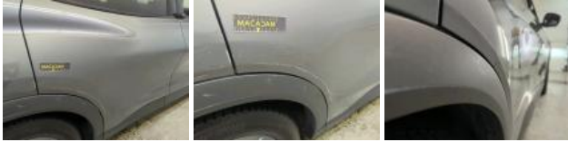
Door FR, Scratch(es), Repair and paint (complete)
