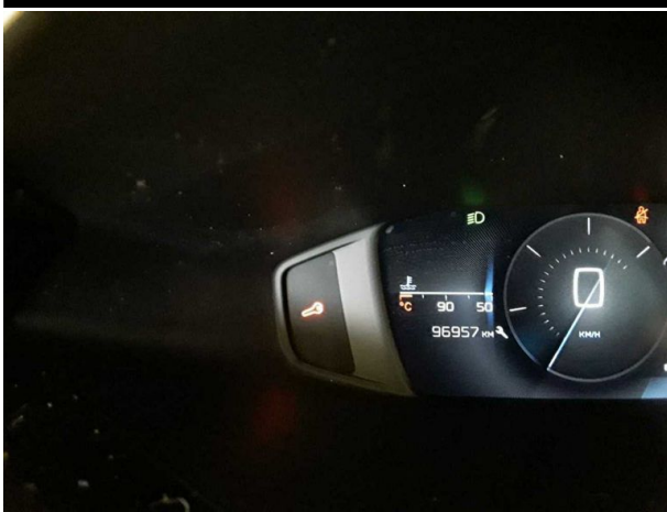
Damage #8: Misc.: Inspection / maintenance - Due - Replace
