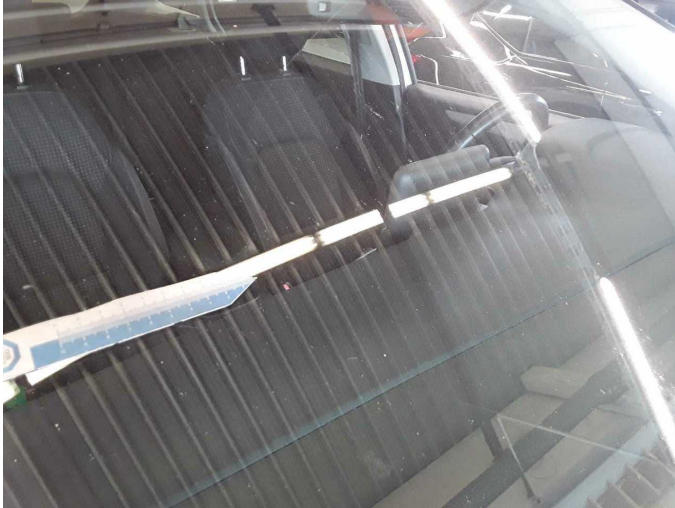
Wear and tear 3: Vehicle glazing: Windscreen - Stone chips - No deduction
