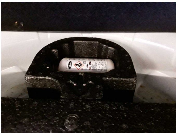
Damage 2: Equipment: Tirefit filler - Expired - Replace
