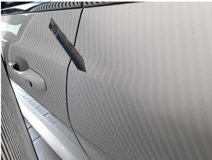
Wear and tear 6: Door - rear left side: Door - dent(s) - Smooth repair work
