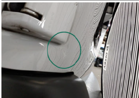
Heckklappe / Kofferraumtür / Unten Links / Delle
