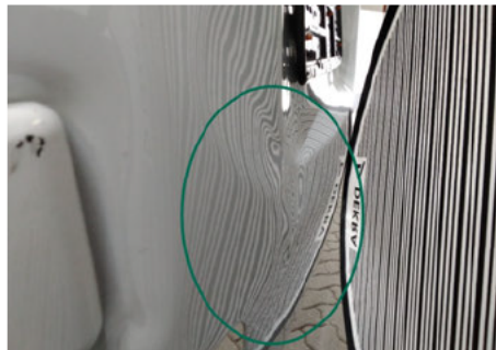
Heckklappe / Kofferraumtür / Unten Links / Delle
