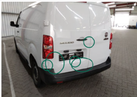
Heckklappe / Kofferraumtür / Unten Links / Delle
