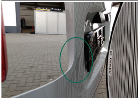
Heckklappe / Kofferraumtür / Unten Links / Delle
