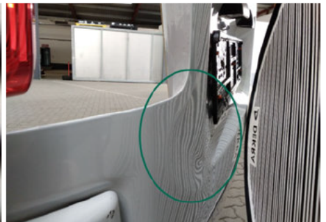
Heckklappe / Kofferraumtür / Unten Links / Delle
