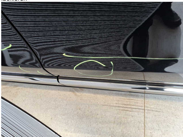
Beschädigung #29: Tür hinten links: Tür - Delle / Lackschaden - lackieren
