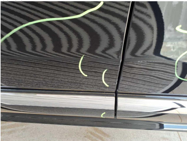
Beschädigung #28: Tür vorn links: Tür - Delle / Lackschaden - lackieren
