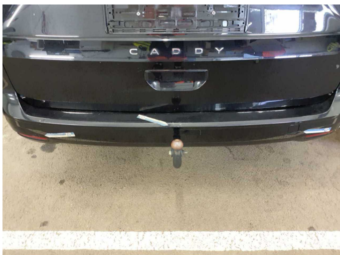
Damage 8: Rear bumper: Rear bumper - Scratch(es) - Paint
