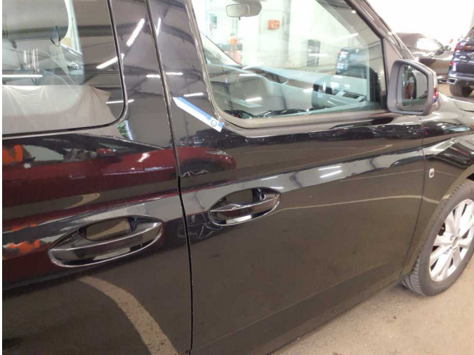
Damage 9: Door - front right side: Door edge (+ Korrosion) - Paint defect - Repair and paint
