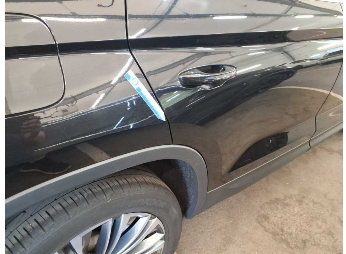
Damage 2: Side panel - rear right side: Side panel - Scratched - Smart repair
