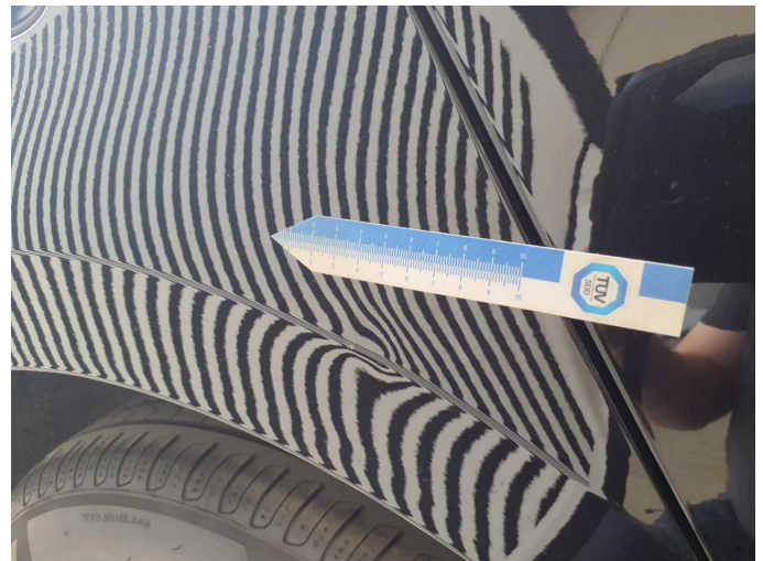
Damage 4: Side panel - rear right side: Side panel - Deformed - Repair and paint
