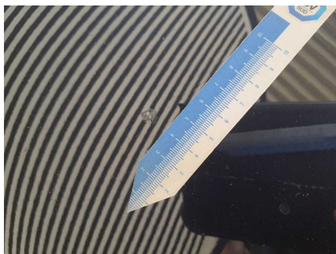
Damage 8: Bonnet: Bonnet (Anätzung) - Paint defect - Repair and paint
