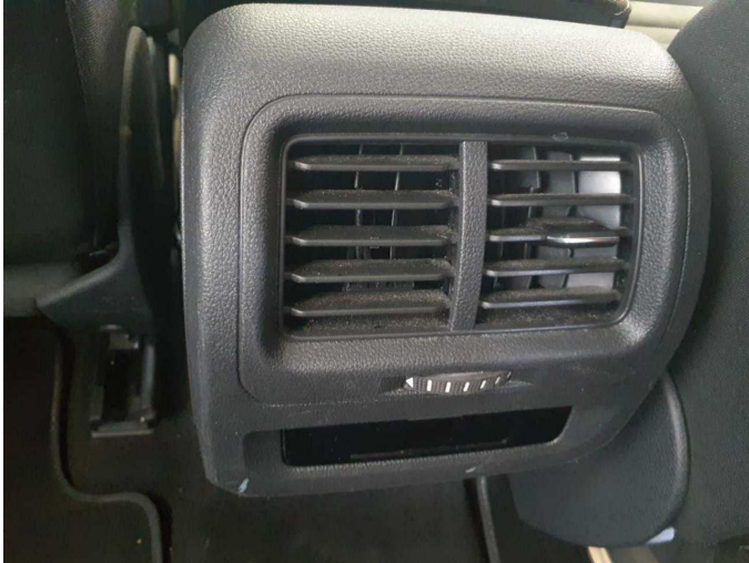
Damage 2: Instrument panel: Air nozzle - centre (Hinten) - Broken / torn - Replace
