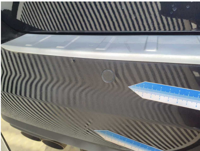
Damage 9: Rear bumper: Rear bumper - Paint defect - Repair and paint
