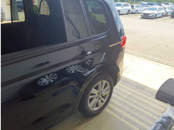
Damage 5: Side panel - rear left side: Side panel (Spachtelmasse eingefallen) - Unprofessionally repaired - Repair and paint
