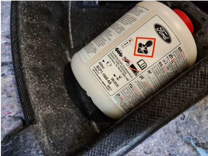
Damage 1: Equipment: Tirefit filler - Expired - Replace
