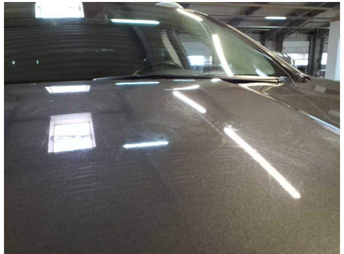
Damage 4: Bonnet: Bonnet - Scratched - Paint
