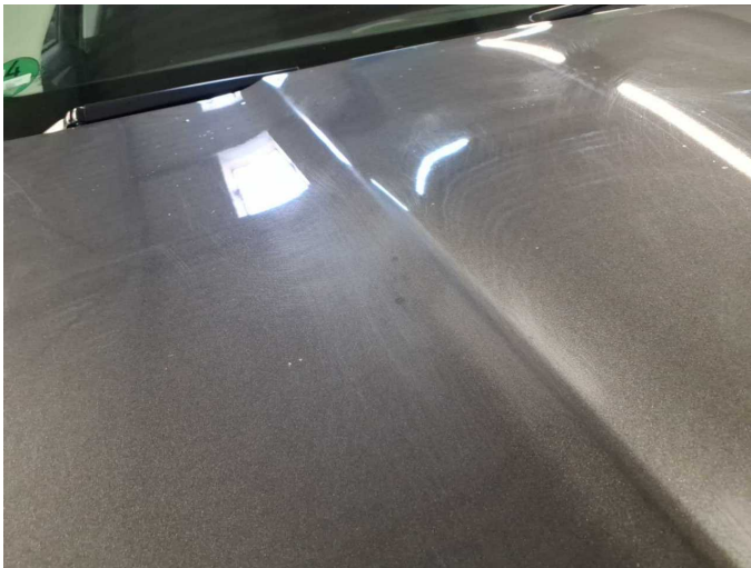
Damage 4: Bonnet: Bonnet - Scratched - Paint
