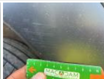
Bumper moulding FL, Scratch(es), Paint
