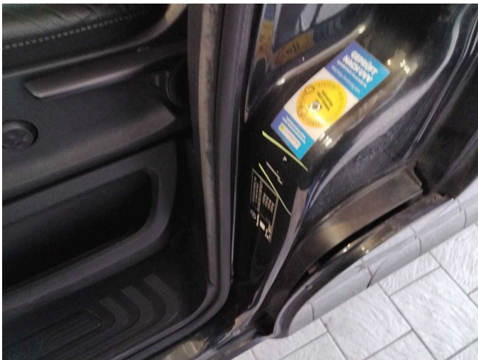
Damage 3: Body: B-pillar - left side - Scratch(es) - Smart repair
