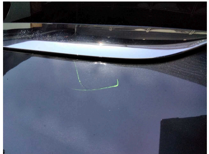
Damage 5: Boot lid / rear door: Boot lid - Dent / paintcoat damage - Repair and paint
