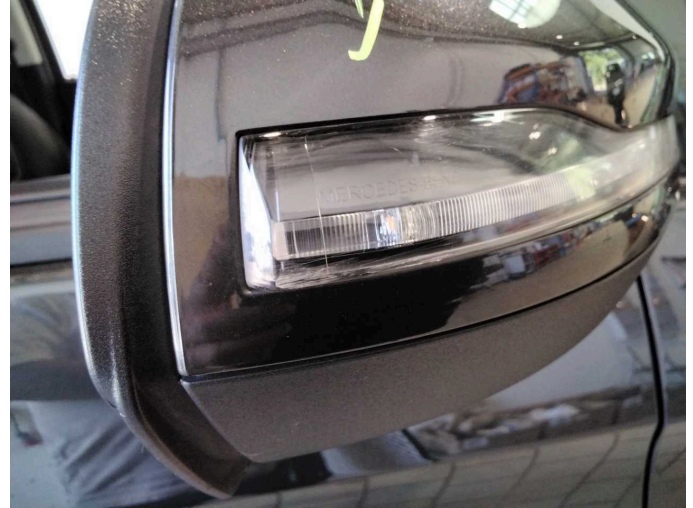
Damage 2: Indicator - front: Mirror - right side - Scratch(es) - Replace
