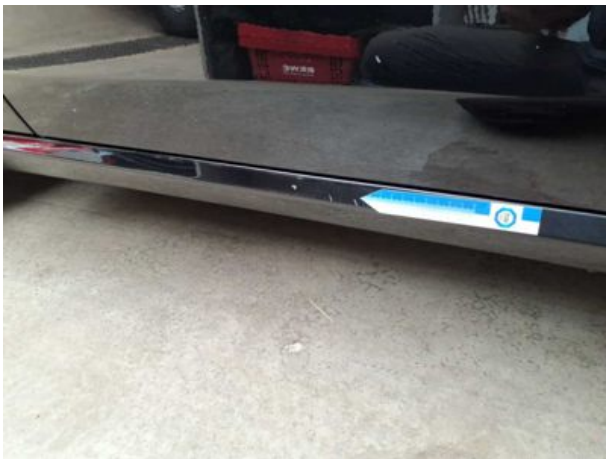
Damage #11: Sill - left side: Trim - Scratch(es) - Smart repair
