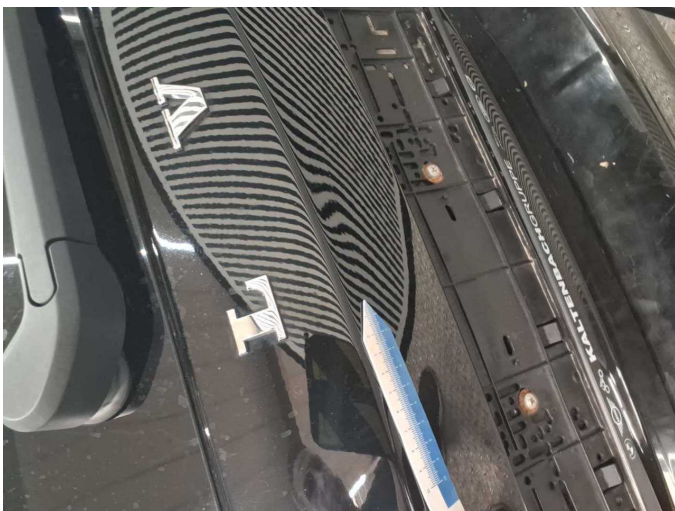
Damage 7: Boot lid / rear door: Boot lid - dent(s) - Smart repair
