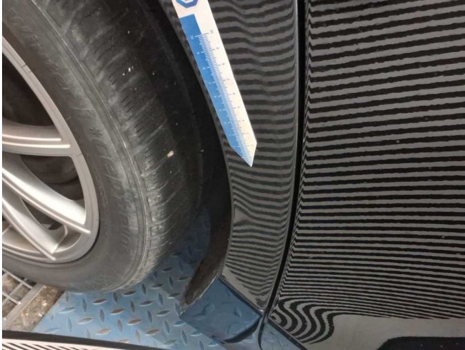
Damage 5: Side panel - rear right side: Elbow - dent(s) - Smart repair
