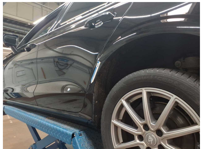
Damage 8: Side panel - rear left side: Elbow - Scratch(es) - Smart repair
