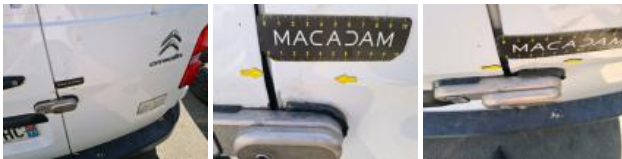
Boot door panel RL, Rust, Paint
