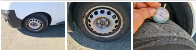
Wheel cover FL, Missing, Replace
