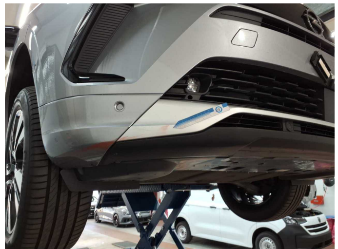
Damage 1: Front bumper: Spoiler - Scratched - Cover / polish
