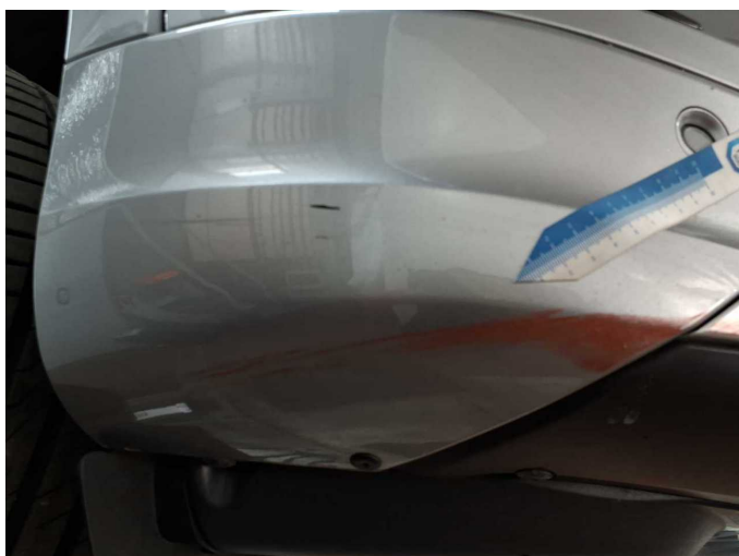
Damage 5: Front bumper: Spoiler (Zierleiste re) - Scratched - Paint
