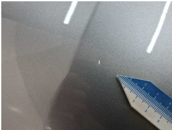
Damage 8: Bonnet: Bonnet - Dent / paintcoat damage - Paint
