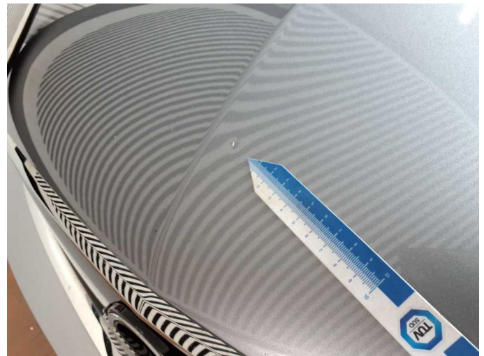
Damage 8: Bonnet: Bonnet - Dent / paintcoat damage - Paint
