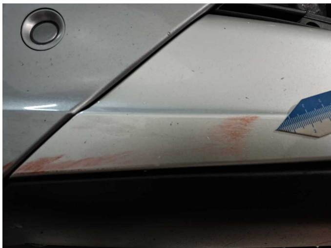
Damage 1: Front bumper: Spoiler - Scratched - Cover / polish
