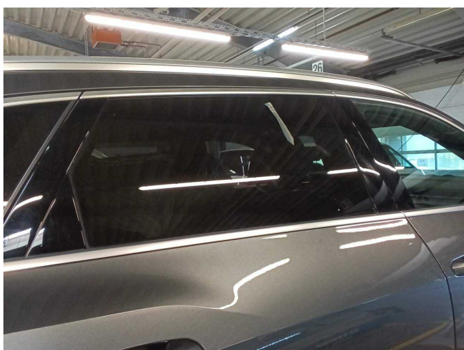
Damage 2: Vehicle glazing: Door glass - rear right side - Scratch(es) - Loss in value
