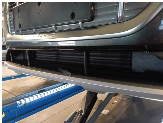
Damage 5: Front bumper: Spoiler - Scratched - Smart repair
