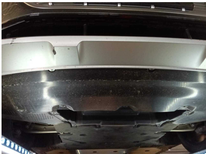
Damage 1: Body: Underbody panelling - Scratched - Replace
