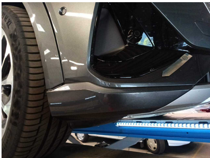
Damage 4: Trim / covers: Trim / covers - Scratch(es) - Smart repair
