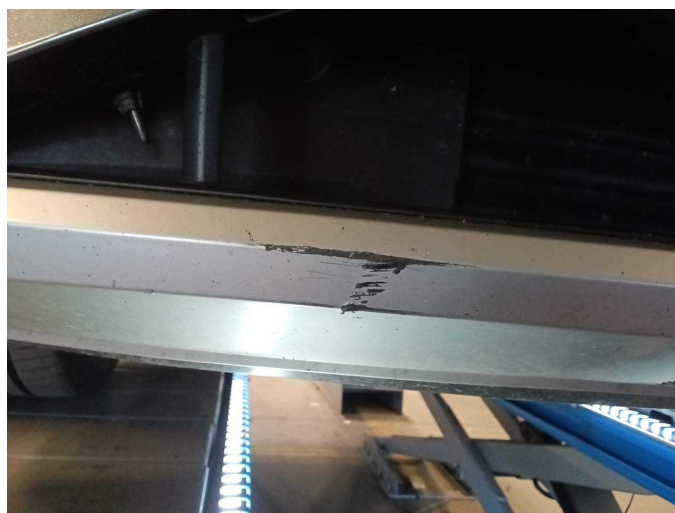
Damage 5: Front bumper: Spoiler - Scratched - Smart repair
