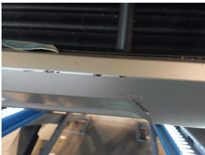
Damage 5: Front bumper: Spoiler - Scratched - Smart repair
