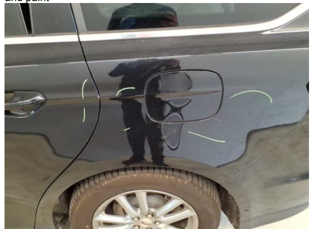
Damage #13: Side panel - rear left side: Side panel - Scratch... - Repair and paint
