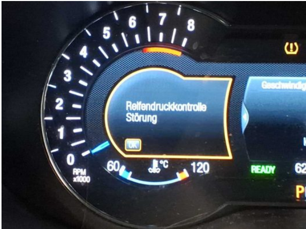
Damage #2: Instrument panel: Indicator light (RDKS brennt) - Differs from the original configuration - Perform diagnosis
