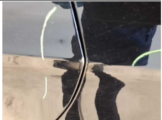
Damage #8: Door - rear left side: Door - Scratched - Repair a... paint
