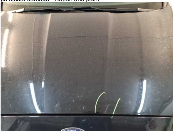
Damage #15: Bonnet: Bonnet - Scratched - Repair and paint
