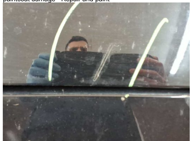
Damage #15: Bonnet: Bonnet - Scratched - Repair and paint
