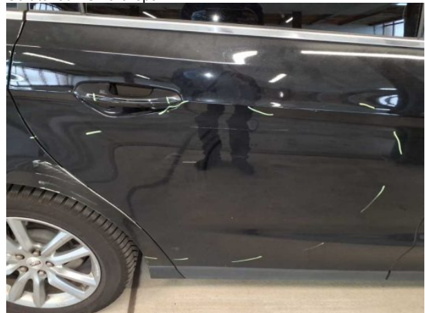
Damage #5: Door - rear right side: Door handle - outside - Scratched - Smart repair
