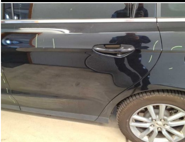
Damage #8: Door - rear left side: Door - Scratched - Repair and paint
