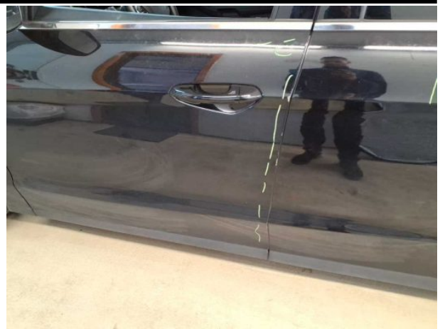
Damage #11: Door - front left side: Door - Scratched - Repair and paint
