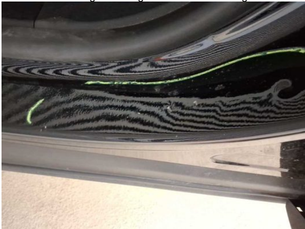
Damage #3: Sill - left side: Sill - Dent / paintcoat damage - Smart repair
