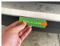
Bumper moulding R, Scratch(es), Paint
