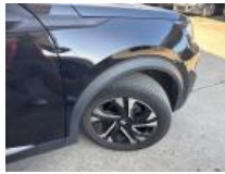
Tyre FL, Out of tolerance, Replace
