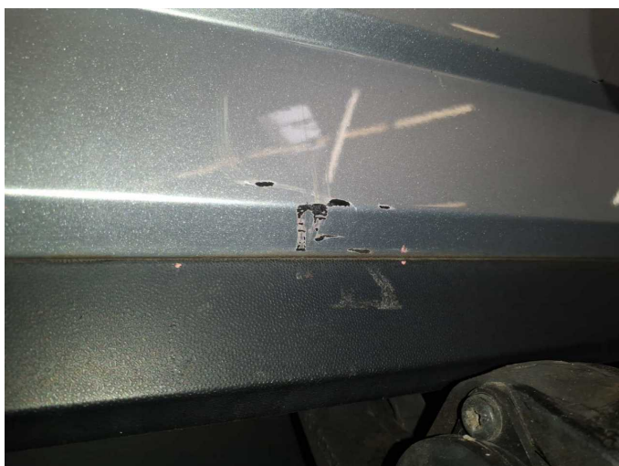
Damage 8: Rear bumper: Rear bumper - Scratched - Paint
