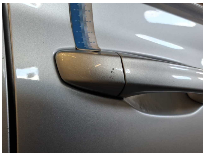
Wear and tear 2: Door - front right side: Door handle - outside (Schlosskappe) - Scratched - No deduction
