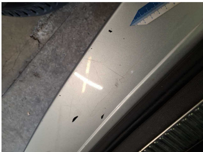
Damage 8: Rear bumper: Rear bumper - Scratched - Paint
