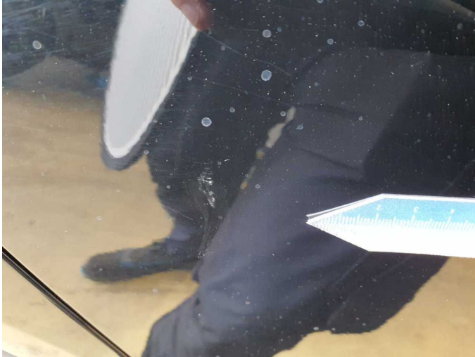
Damage 1: Door - rear right side: Door - Dent / paintcoat damage - Smart repair
