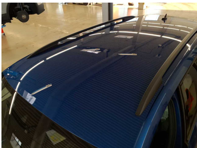
Damage 11: Roof: Roof (Einätzungen + Dellen) - Paint defect - Repair and paint
