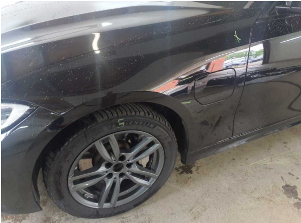
Damage #1: Mudguard - left side: Mudguard - left side - dent(s) - Smooth repair work
