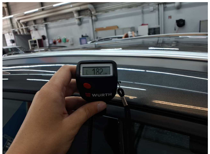
Repainting 1: Roof rail - right side
