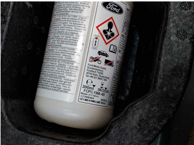
Damage 1: Equipment: Tirefit filler - Expired - Replace
