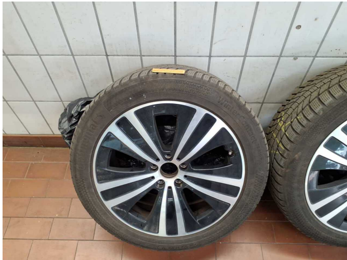
Damage 4: 2nd wheel set: 2 tyres (4mm) - Does not meet the leasing specifications - Replace
