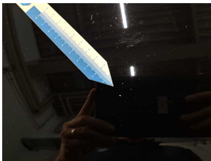
Damage 7: Bonnet: Bonnet - Stone chips - Paint
