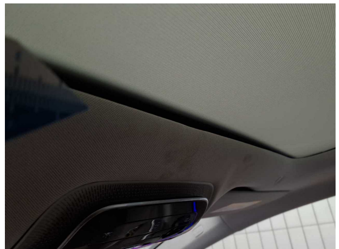
Damage 1: Trim / covers: Roof lining - Damaged - Smart repair
