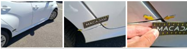
Door FR, Bad repair, Paint
