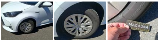
Wheel cover FL, Broken, Replace
