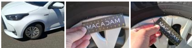
Tyre RL, Out of tolerance, Replace
