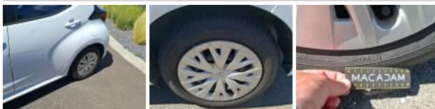
Wheel cover RL, Broken, Replace
