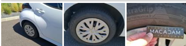
Wheel cover RR, Broken, Replace
