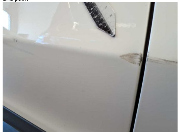
Damage #10: Door - rear right side: Door - Dent / paintcoat damage - Repair and paint
