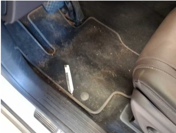
Damage #1: Trim / covers: Floor mats - Holes - Replace
