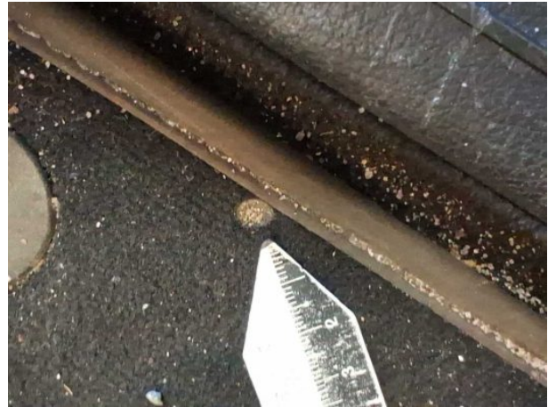
Damage #1: Trim / covers: Floor mats - Holes - Replace
