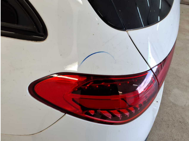
Damage #3: Side panel - rear left side: Side panel - Scratch(es) - Cover / polish
