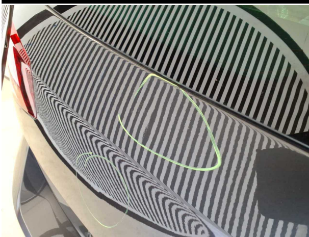
Damage #4: Boot lid / rear door: Boot lid - dent(s) - Smooth repair work
