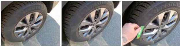
Tyre RR, Out of tolerance, Replace
