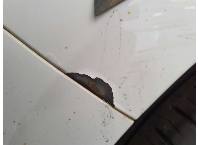
Damage 9: Side panel - rear right side: Side panel (Lack blättert ab + Korrosion) - Paint defect - Repair and paint
