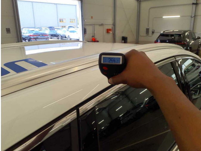
Repainting 2: Roof rail - right side
