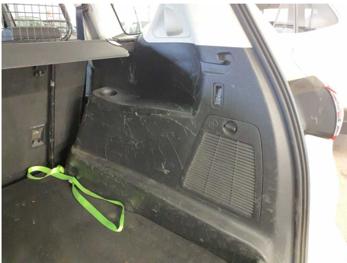
Damage 3: Trim / covers: Cargo area - lining - right side - Scratch(es) - Loss in value
