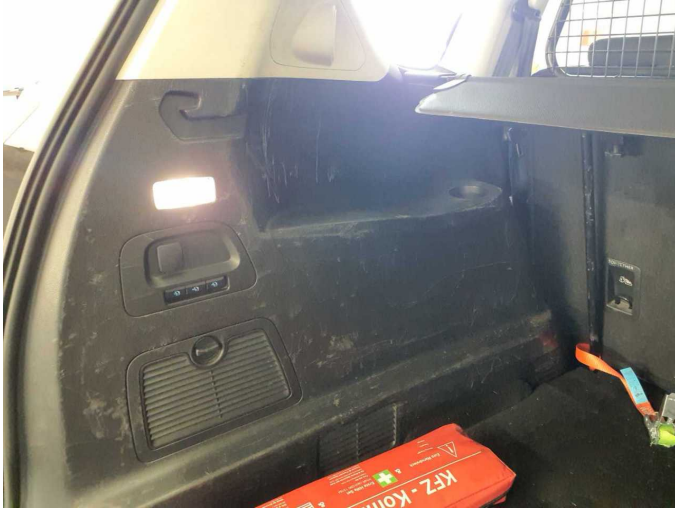
Damage 4: Trim / covers: Cargo area - lining -left side - Scratch(es) - Loss in value
