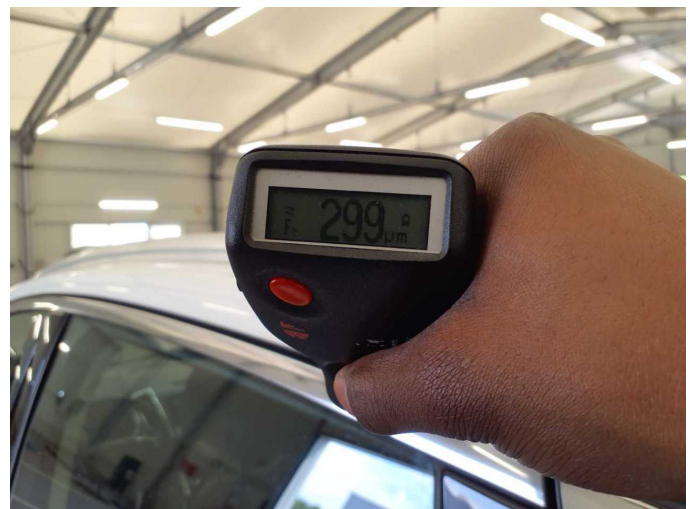
Repainting 1: Roof rail - left side
