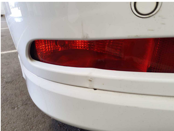
Damage 10: Rear bumper: Rear bumper - Dent / paintcoat damage - Repair and paint
