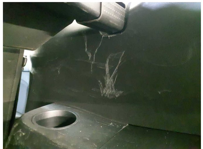
Damage 3: Trim / covers: Cargo area - lining - right side - Scratch(es) - Loss in value
