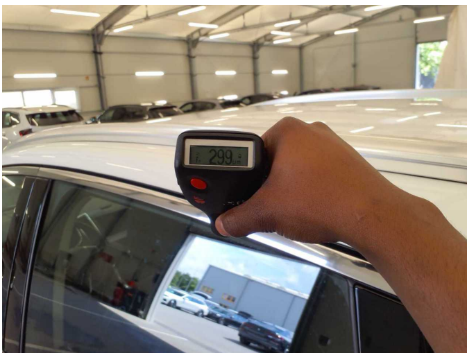
Repainting 1: Roof rail - left side
