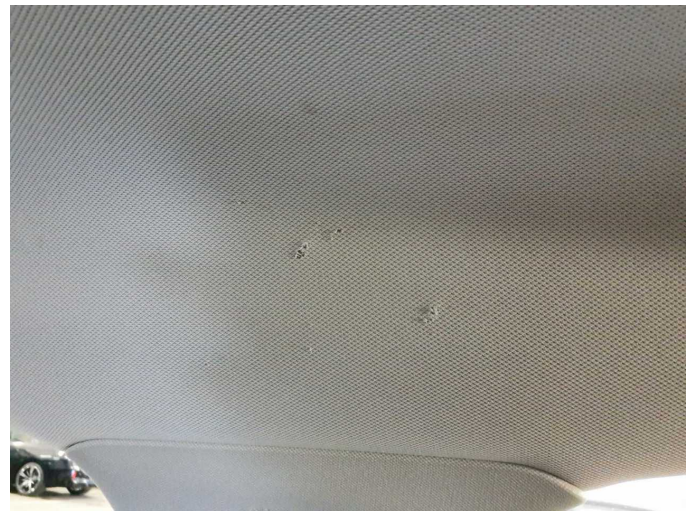
Damage 6: Trim / covers: Roof lining - Holes - Smart repair
