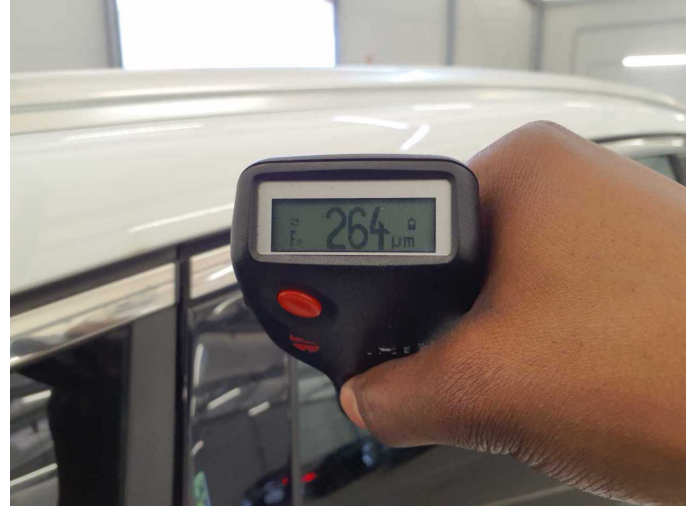
Repainting 2: Roof rail - right side
