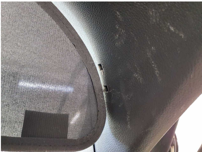
Missing part 1: Interior: Boot cover / roller cover (Halierung) - Missing - Replace
