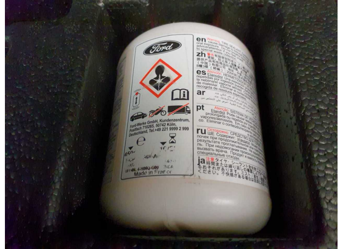
Damage 2: Equipment: Tirefit filler - Expired - Replace
