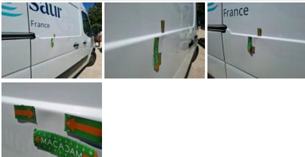
Side panel moulding R, Unclapsed, Dismount/Mount
