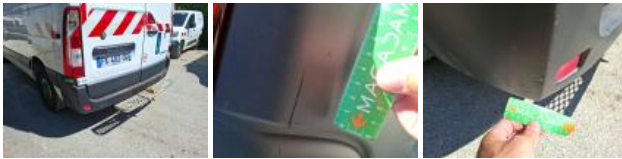
Internal boot lining L, Broken, Replace
