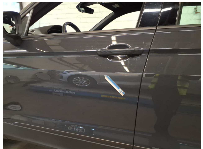
Damage 3: Door - front left side: Door - dent(s) - Smooth repair work
