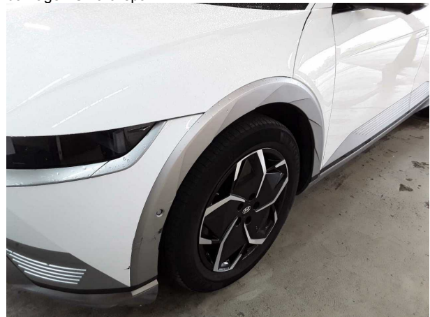
Damage #3: Mudguard - left side: Wheel well extension - Scratched - Replace
