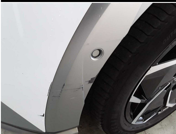
Damage #3: Mudguard - left side: Wheel well extension - Scratch... - Replace
