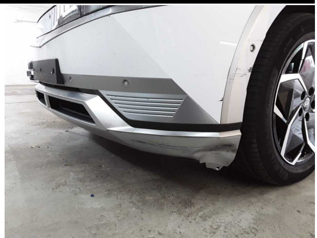
Damage #4: Front bumper: Spoiler - Damaged - Replace
