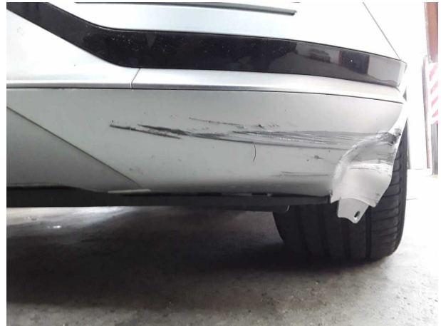
Damage #4: Front bumper: Spoiler - Damaged - Replace
