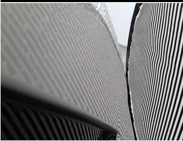
Damage #8: Side panel - rear left side: Side panel - Dent / paintcoat damage - Repair and paint
