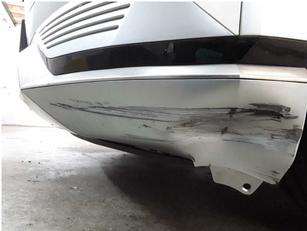
Damage #4: Front bumper: Spoiler - Damaged - Replace
