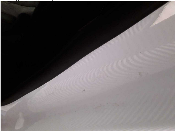
Damage #2: Side panel - rear left side: Sill - Dent / paintcoat damage - Smart repair
