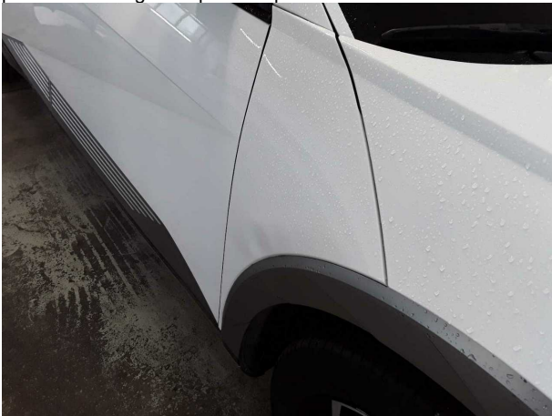
Damage #9: Mudguard - right side: Mudguard - right side - Deformed - Replace
