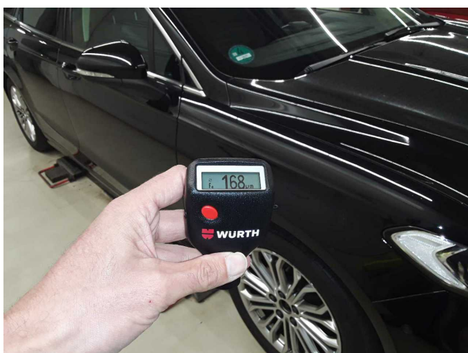
Mudguard - right side: 168 µm
