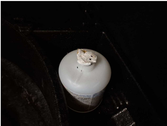
Damage 2: Equipment: Tirefit filler - Empty - Replace
