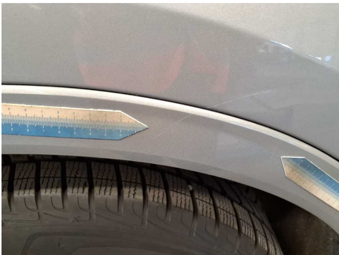
Damage 3: Side panel - rear left side: Wheel well extension - Scratch(es) - Smart repair
