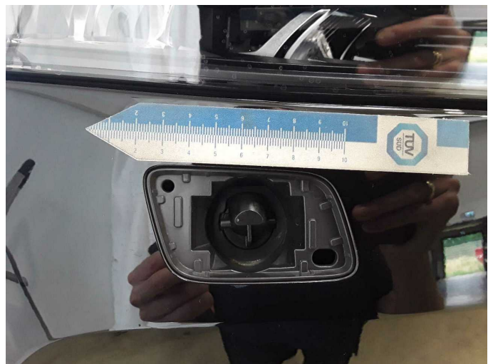
Damage 1: Headlight: Headlight cleaning nozzle - right side (Kappe fehlt) - Missing - Replace
