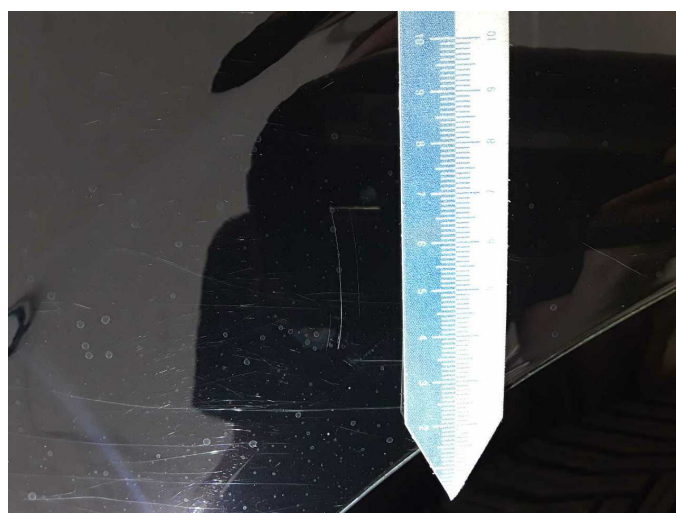
Damage 5: Mudguard - right side: Mudguard - right side - Scratch(es) - Paint
