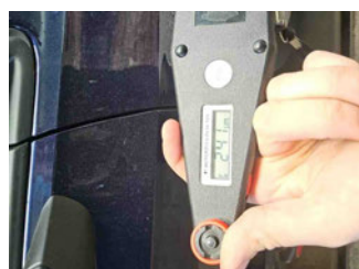
Paint thickness Door FR
