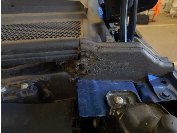
Damage 1: Cab: Insulation lining - Damage caused by marten / rodent - Replace
