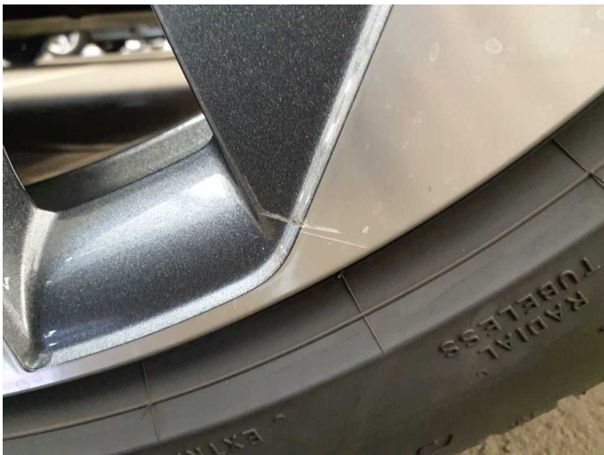
Damage 5: Wheel / tyres: Alloy rim - rear left side - Scratched - Loss in value
