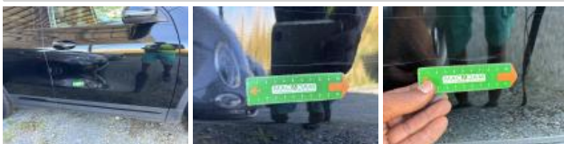
Door RR, Dent(s), Repair and paint (complete)
