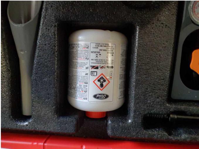
Damage 2: Equipment: Tirefit filler - Expired - Replace
