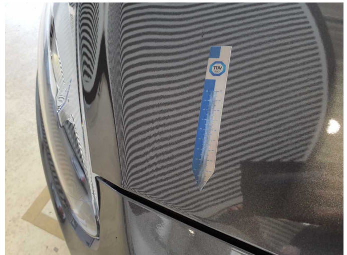
Damage 4: Bonnet: Bonnet (Spachtelmasse eingefallen) - Unprofessionally repaired - Repair and paint
