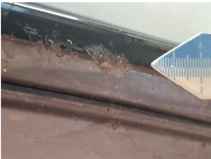
Damage 6: Front bumper: Spoiler - Scratched - Replace
