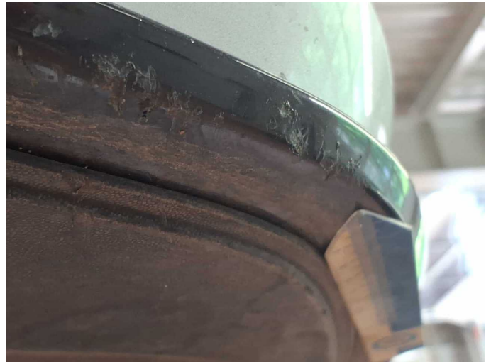
Damage 6: Front bumper: Spoiler - Scratched - Replace
