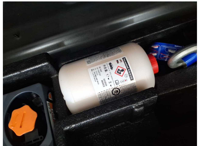
Damage 1: Equipment: Tirefit filler - Expired - Replace
