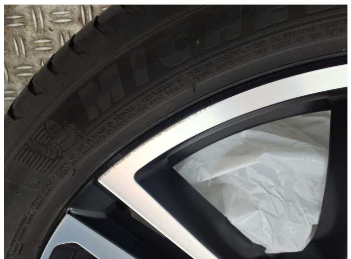
Damage 7: 2nd wheel set: 2 alloy rims - Scratch(es) - Loss in value
