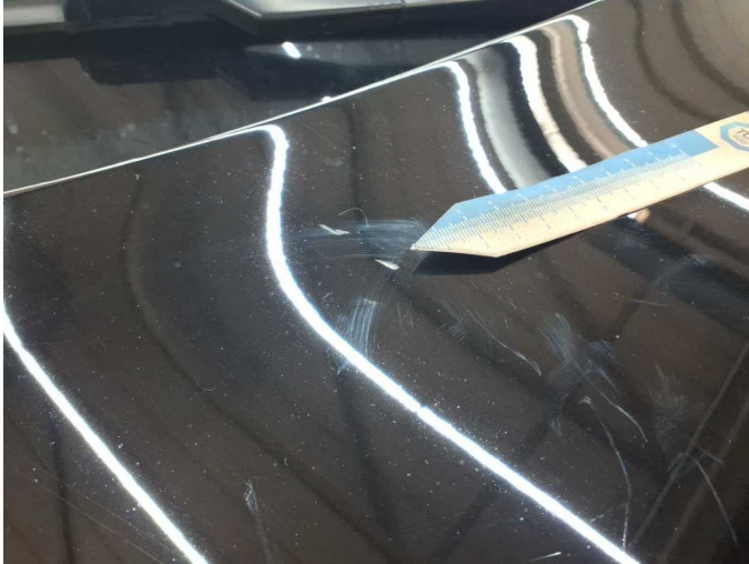
Damage 11: Bonnet: Bonnet - Scratch(es) - Paint
