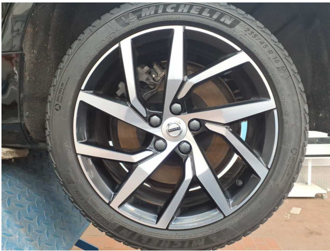
Damage 4: Braking system: Brake discs and pads - rear (Freibremsen) - Corrosion
