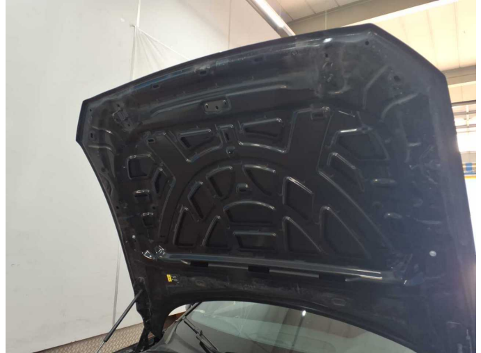
Damage 6: Bonnet: Insulation lining - Missing - Replace
