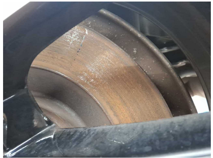
Damage 4: Braking system: Brake discs and pads - rear (Freibremsen) - Corrosion
