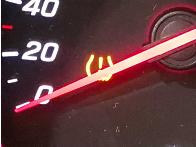
Damage 2: Instrument panel: Indicator light (Reifendruckkontrolle) - on - Perform diagnosis
