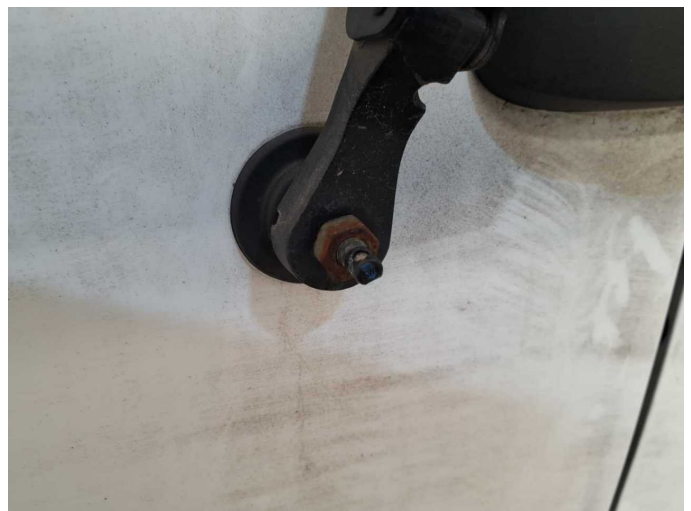
Damage 1: Screen cleaning: Wiper arm - rear (Blende) - Missing - Replace
