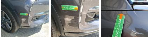
Bumper moulding FR, Scratch(es), Replace
