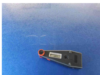
Paint thickness Roof
