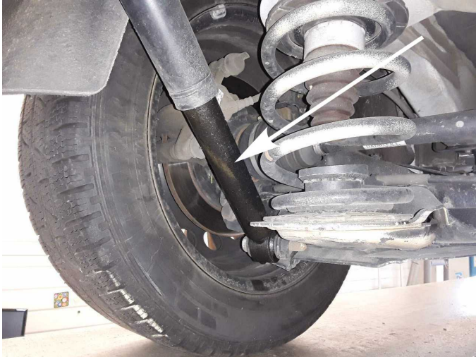
Damage 6: Rear axle: Shock absorber - left side - Leaking - Replace
