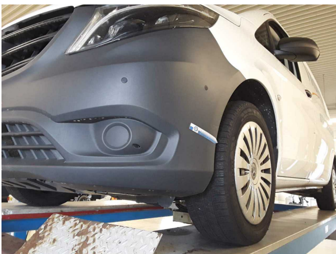
Wear and tear 1: Front bumper: Front bumper - Scratch(es) - No deduction
