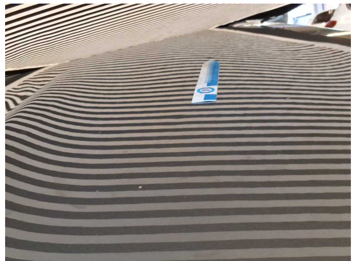
Damage 9: Bonnet: Bonnet - Dent / paintcoat damage - Paint
