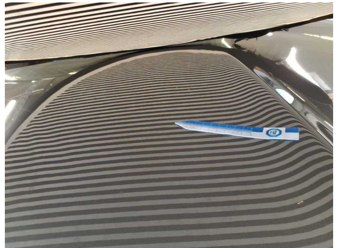
Damage 9: Bonnet: Bonnet - Dent / paintcoat damage - Paint
