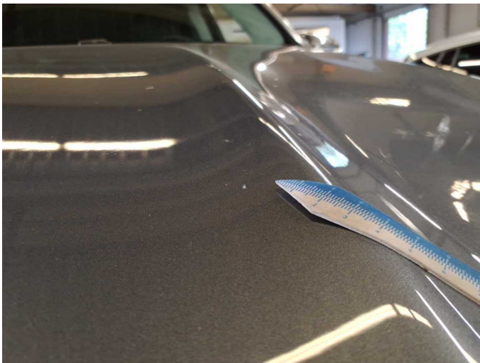
Damage 9: Bonnet: Bonnet - Dent / paintcoat damage - Paint
