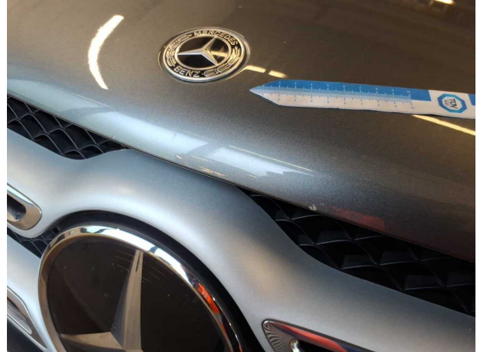
Damage 9: Bonnet: Bonnet - Dent / paintcoat damage - Paint
