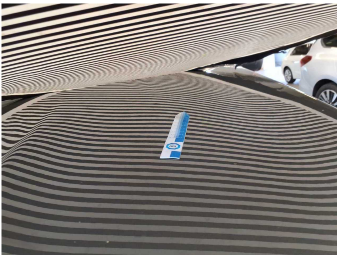
Damage 9: Bonnet: Bonnet - Dent / paintcoat damage - Paint
