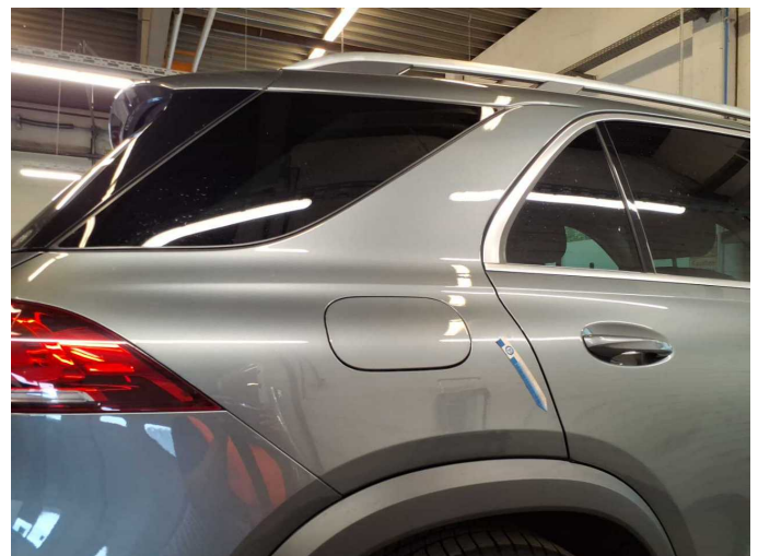
Damage 1: Side panel - rear right side: Side panel - dent(s) - Smooth repair work
