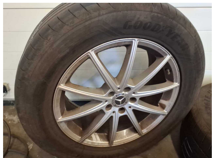
Damage 8: 2nd wheel set: 1 tyre (nicht fahrbereit) - Leaking - Replace
