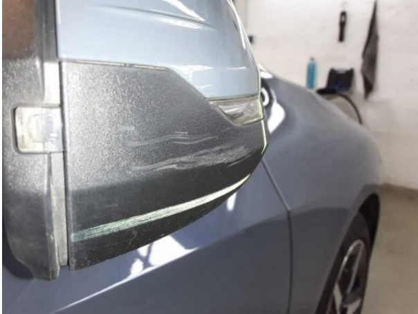
Damage #4: Wing mirror - left side: Mirror housing - Scratched - Loss in value
